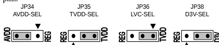
Figure 4. Setting of jumper pins when using the power supply connector.
