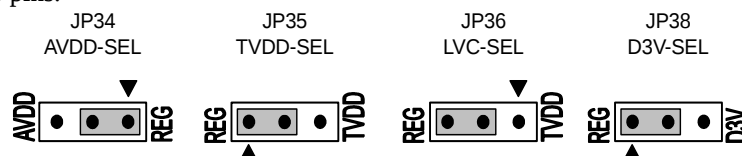
Figure 3. Setting of jumper pins when using the regulator at the all power supply lines.
